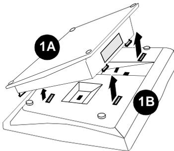
Remove the desktop stand (1A) from the bottom of the telephone (1B). Push inward on the top of the stand until you can lift the top of the stand from the tab slots on the telephone.
