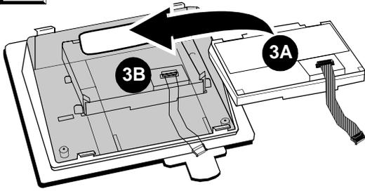
Install the module (3A) in the desktop stand (3B). Push down until you hear the module snap in place.
