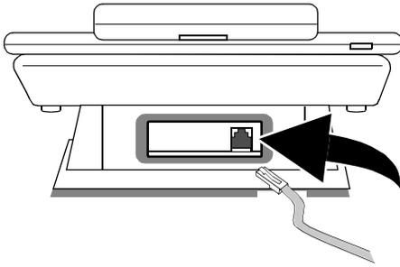
Connect the analog adjunct such as a modem, fax machine, or analog telephone to the module.
