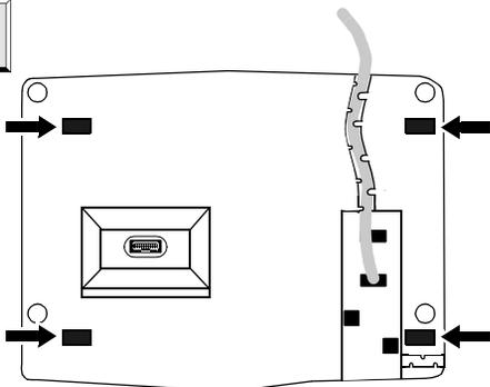
Replace the stand and module by lowering the desktop stand onto the bottom of the telephone. The tabs on the stand must snap into the appropriate slots on the bottom of the telephone. (These slots are marked with arrows in the accompanying drawing on the left.)
