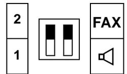
**2. IF THE OPTION SWITCH ON THE LEFT IS SET TO 1, YOU MUST SET THE OPTION SWITCH ON THE RIGHT TO EITHER FAX OR [Speakerphone Icon]**
