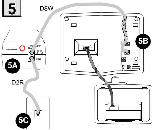
Connect the stand-alone local auxiliary power supply (5A). With the D8W cord, connect the auxiliary power supply (the PHONE jack) to the Line jack on the telephone (5B). Then, connect the power supply (the LINE jack on the power supply) to a wall jack (5C).
