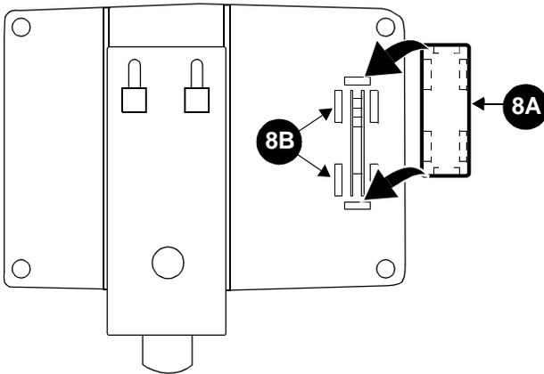
The desktop stand has slots in which you can store the cover (8A) you removed from the module opening (see Step 2) in case you need to reinsert the cover at a later time. (8B shows the location of the storage area.) Snap the tabs on the cover into the slots provided on the desktop stand.
