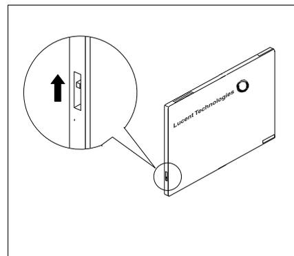
**4** To insert the PC Card, hold it with the label facing to the right, and slide it gently into one of the PC Card slots on the processor module. When inserted properly, the PC Card projects about 1-5/8" (4 cm) from the module.
