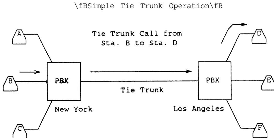
In special cases, tie trunks are used to join one PBX directly to another PBX. This may occur if multiple PBXs serve a single-customer at a single location. A typical example would be a corporate headquarters consisting of several buildings, each housing a separate division, co-located in a campus setting on a single premises. This is sometimes called a "back-to-back" connection.
