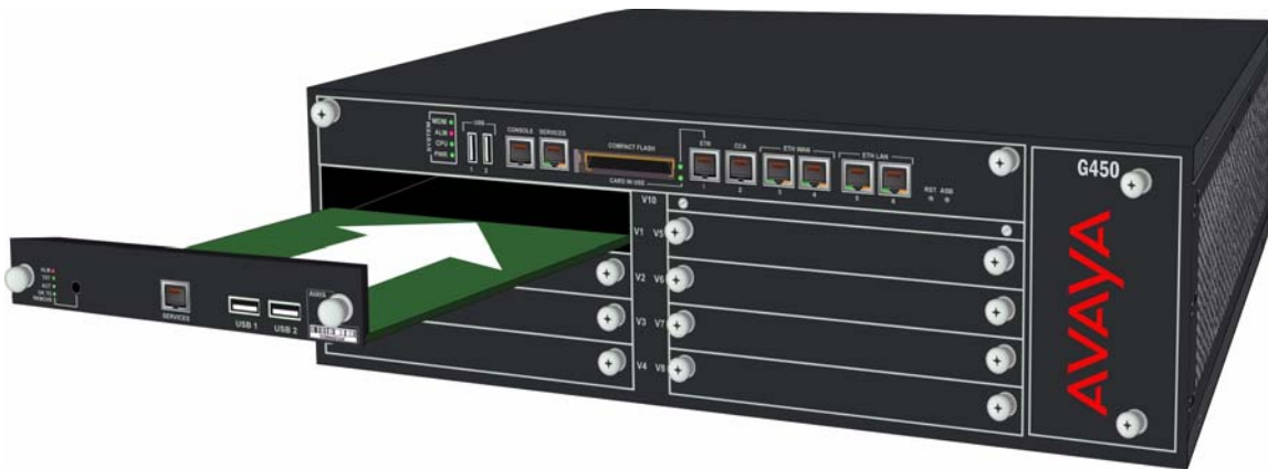
Figure 7: Inserting the S8300 Server module.
