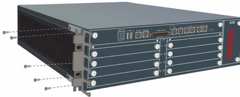
Figure 3: Attaching a mounting bracket with cable guides
