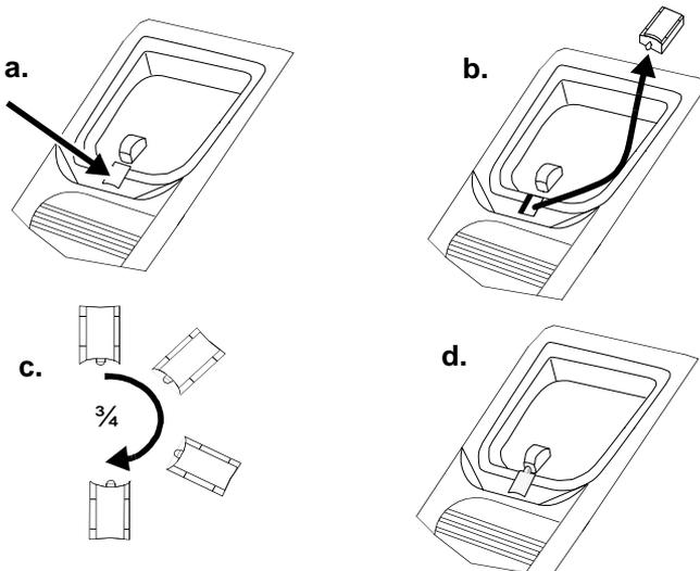
**FIGURE 6** Removing, Rotating, and Replacing the Handset Retainer
