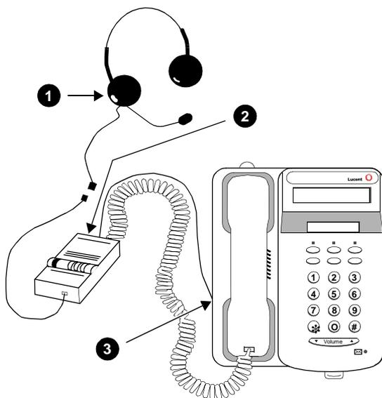
**FIGURE 2 The Headset Attached to a 6402D Telephone**
